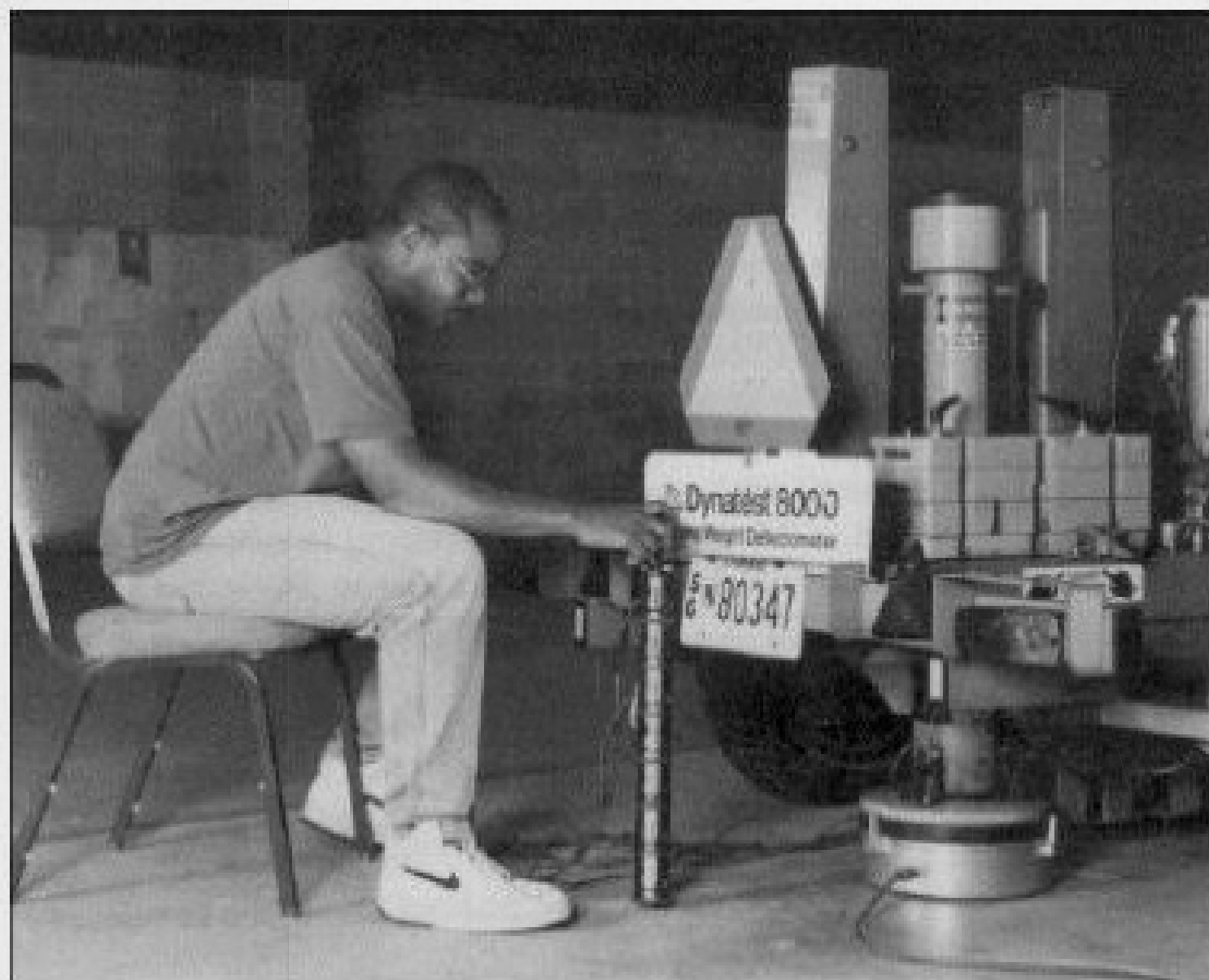
Relative calibration of all of the FWD deflection sensors. Photo Courtesy of PennDOT.
